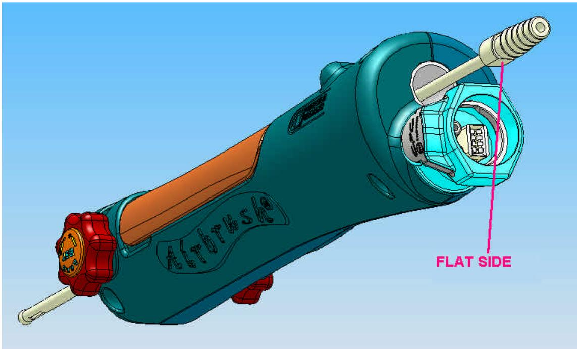
7. Once the inner cannula is firmly seated and snapped into position, slide the matching outer cannula over the inner cannula with the pin oriented in the center of the trigger until the outer cannula hub fits over the mount and rotate the then pin towards the rate knob to secure it.
