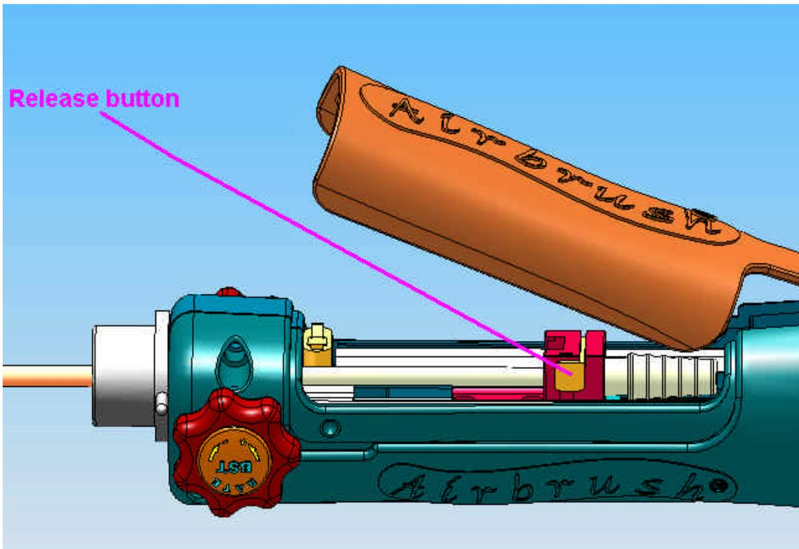
11. At any time the inner cannula can be “popped” out by pointing the outer cannula up and pressing the cannula release button at the back of the instrument by first putting the carriage in the **cannula changing position**.
